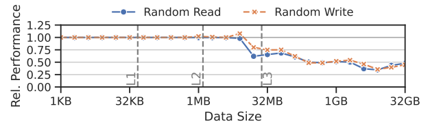
Figure 5: Performance of random memory reads and writes in an SGX enclave relative to plain CPU. In the cache, random access performance is equal. Random accesses to main memory are significantly slower in SGXv2.
