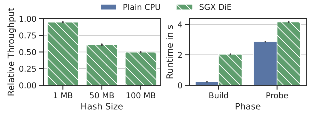
Figure 4: Left: Throughput of a single-threaded hash join with data and execution inside an SGXv2 enclave (DiE) relative to plain CPU. Join performance with large hash tables suffers from random access overhead. Right: Comparison of join phase runtimes at 100 MB hash size. The slowdown of the build phase inside the enclave is significant.
