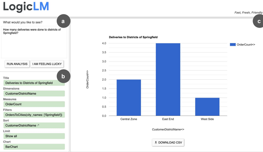
Figure 4: The LogicLM UI displays: (a) a Query Input Panel for user requests; (b) an OLAP Config Panel showing the LLM-generated OLAP configurations, with options for interactive adjustments; and (c) a visualization of the query results.
