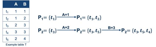
Figure 4: Sequence of the naive multi-key partitioning
