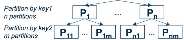
Figure 3: Hierarchical partitioning for two keys
