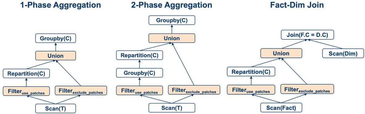
Figure 8: Patched query plans after applying the PatchIndex optimization rule (added operators highlighted)
