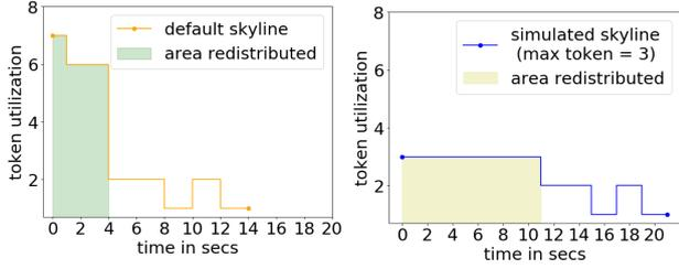
**Figure 7: Redistributed section between the Ground truth (left) skyline and simulated (right) skyline. The simulator reallocates work with fewer resources. To preserve area, the reallocated portion in the simulated skyline takes more than twice as long, when allocated a little less than half as many tokens.**
