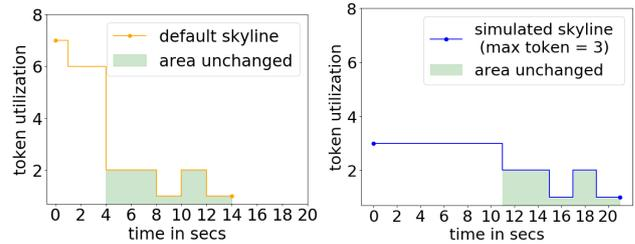
Figure 6: Unchanged section between the Ground truth (left) skyline and simulated (right) skyline.
