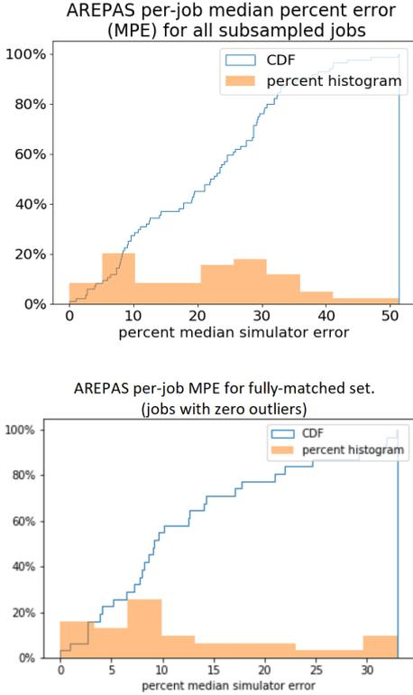
**Figure 13: AREPAS accuracy against the ground truth: median error for jobs with non-anomalous behavior is 9.2%.**
