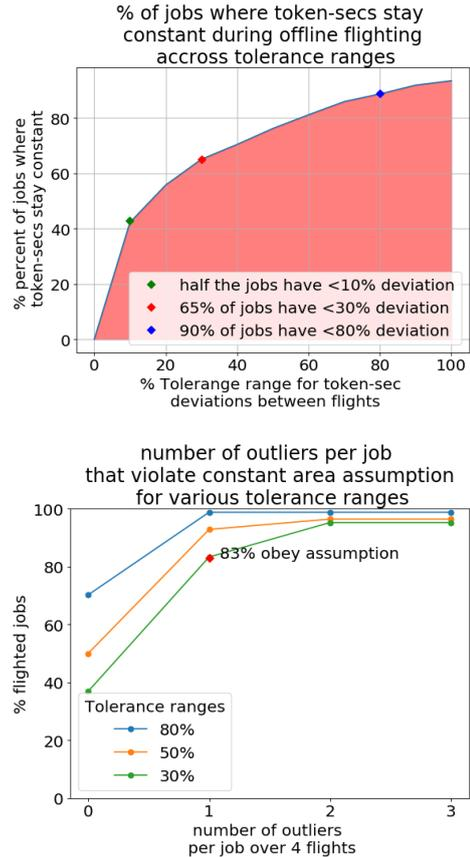
Figure 12: Validating constant resource allocation area assumption: 83% jobs uphold the assumption within a tolerance of up to 30% and with 1 or fewer outliers.
