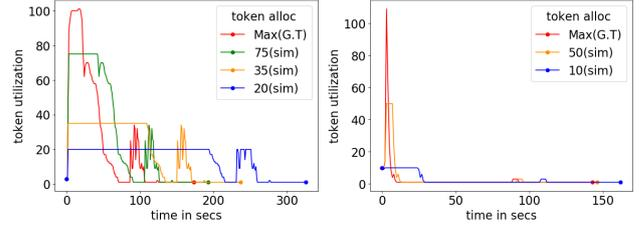
**Figure 8: Flatter jobs (left) lose significant performance as soon as the token allocation is decreased, while peaky jobs (right) can tolerate a significant loss of resource allocation before they lose performance. G.T, that is, Ground Truth, denotes the starting skyline for the simulations.**
