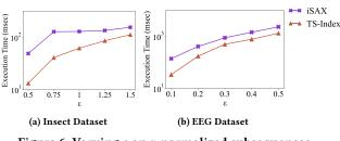
Figure 6: Varying  $\epsilon$  on z-normalized subsequences.
