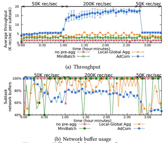
Figure 4: Effect of change in data rate.
