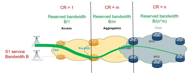
**Figure 4: Convergence ratio (CR) in IP-RAN networks.**
