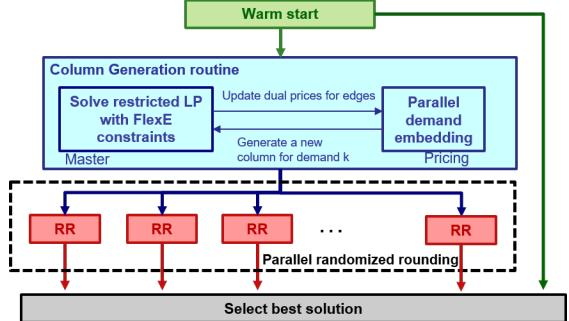
Figure 5: Algorithmic framework to solve *FlexE-CG*.
