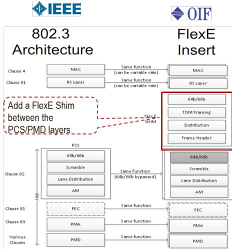
**Figure 1: Extension of IEEE 802.3 to support Flex Ethernet.**
