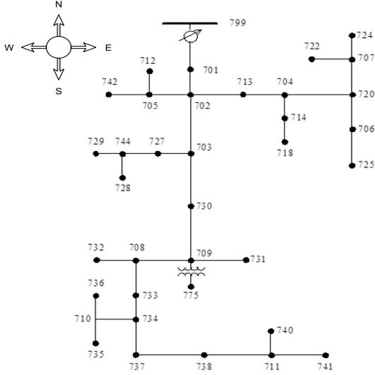
Figure 1: IEEE 37 node radial test network.
