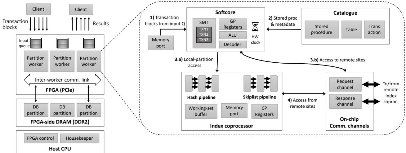
**Figure 2: Architecture of BionicDB and the processing flow within a partition worker: 1) ingesting an input transaction block from memory, 2) fetching stored procedure code and metadata from the catalogue, 3.a) dispatching an index operation to the local index coprocessor 3.b) or to a remote site through the on-chip communication channels and 4) processing an index operation from remote workers.**
