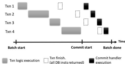
**Figure 8: Transaction interleaving and 2 phase execution.**
