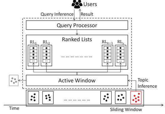
**Figure 4: The architecture for  $k$ -SIR query processing**
