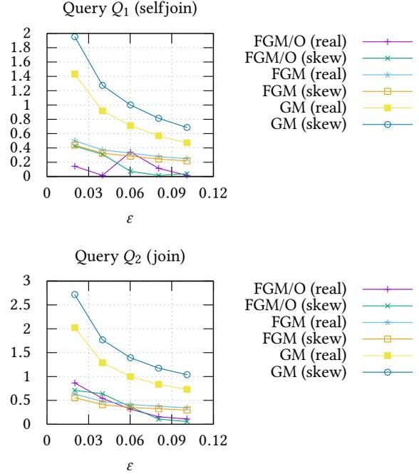
**Figure 6: Communication cost for queries  $Q_1$  (top) and  $Q_2$  (bottom), over varying accuracy  $\varepsilon$ . For each protocol, two curves are shown, one for the real dataset and one for the skewed dataset. For both plots:  $k = 27$ ,  $D = 7000$ , turnstile model ( $T_W=4\text{hrs}$ )**
