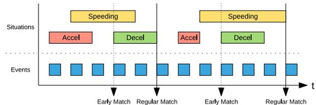
Figure 1: Detecting aggressive driving with situations
