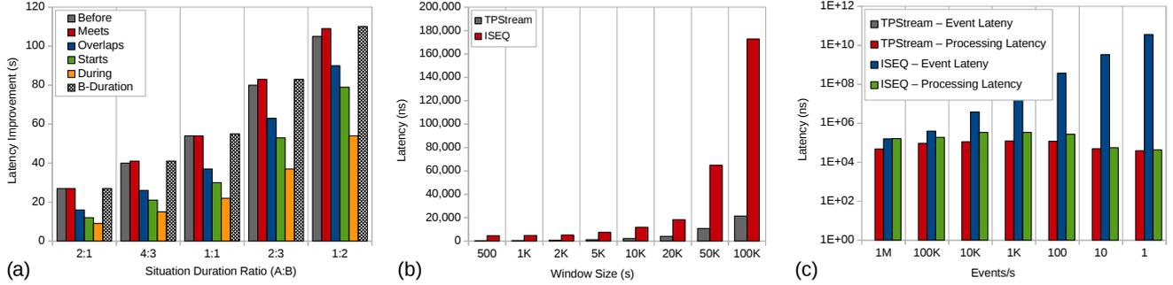
**Figure 7: (a) application time latency gain per temporal relation and comparison of result latency (b) under maximum possible throughput as a function of the window size, (c) under varying event rates with a fixed size window**
