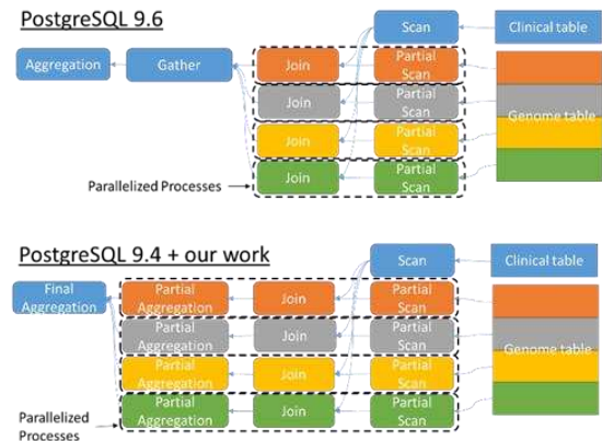
Figure 5: Parallelized query plan
