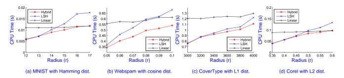
Figure 2: Comparison of CPU Time (s) for a query set between hybrid search (Hybrid), LSH-based search (LSH), and linear search (Linear) on 4 data sets using different metric distances.
