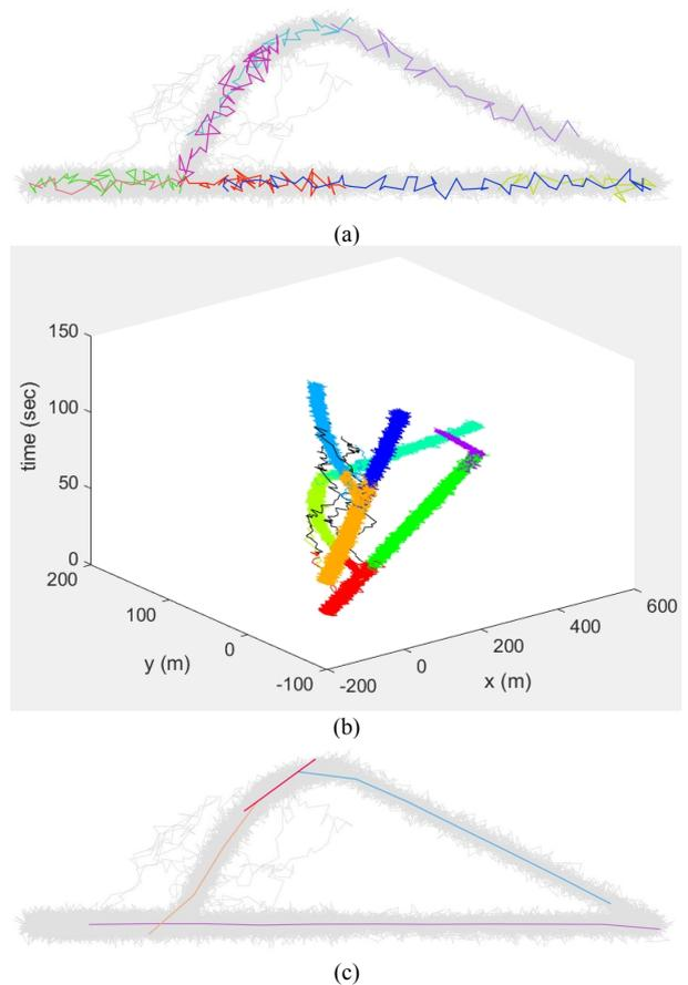
**Figure 6. Visualization of the clusters' representatives provided by: (a) S<sup>2</sup>T-Clustering in (a) 2D and (b) 3D, (c) TRACLUS, when applied to the entire SMOD consisting of 8 patterns.**
