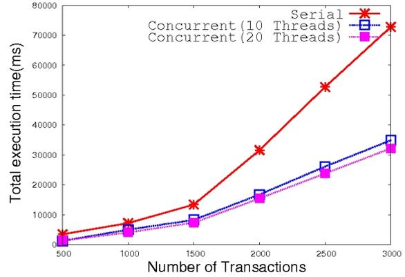
Figure 11: Total execution time for Serial and Concurrent execution of transactions.
