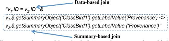
The expression combines both data- and summary-based join operators. As will be discussed in Section 5 and based on the available indexes and statistics, the query optimizer may decide to join the tuples based on the data values and then applies a summary-based selection operator, i.e.,  $(\mathcal{S}(R \bowtie S))$ . Alternatively, it may join the tuples based on the summary objects and then applies a standard selection operator  $(\rho(\mathcal{J}(R, S)))$ .
