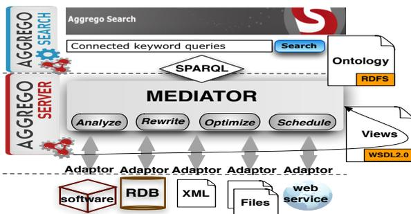
Figure 6: Architecture of AGGREGO toolbox
