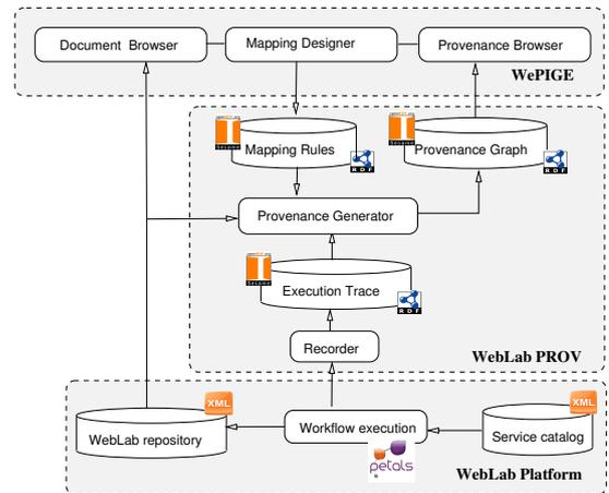
Figure 2: Architecture of WebLab PROV
