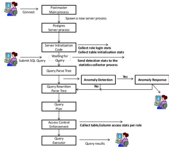
Figure 1: Anomaly Detection and Data Collection Hooks in PostgreSQL.
