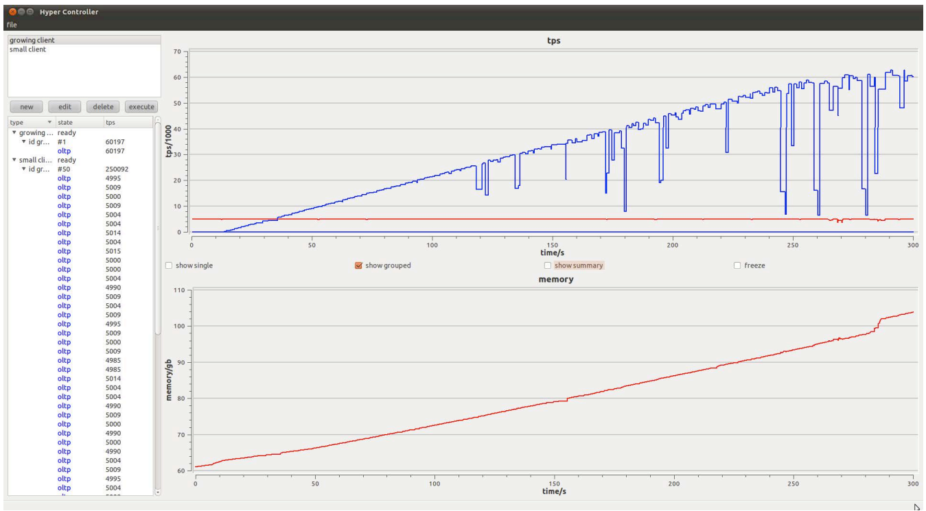
Figure 4: Screenshot displaying the management component of our approach. The diagram in the top-right shows a live view of the transaction throughput of each tenant. Note that the constantly rising transaction rate of the blue tenant does not influence the other 50 instances pictured in red.
