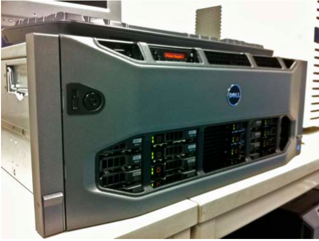
Figure 2: A commodity server (relevant equipment details are listed in Appendix A) capable of a combined TPC-C like transaction throughput of up to 2 million transactions per second. Notice the keyboard on top of the machine for scale.
