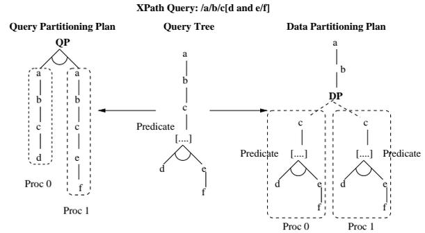
Figure 4: Query and data partitioning plans.
