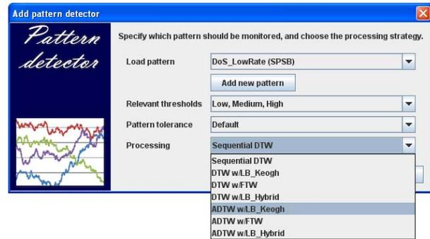
Figure 5: Setup dialog for patterns: allows loading or specifying of patterns, and setting the desired level of sensitivity via the alert threshold and its tolerance via the DTW band. Additionally, the underlying query processing algorithm can be chosen.
