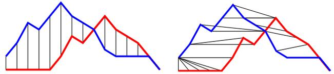
**Figure 4: Euclid (left) vs. DTW (right):** black vertical lines indicated how Euclidean compares the top blue pattern to its shifted counterpart at the bottom (red), and how DTW matches corresponding parts in the patterns through stretching.
