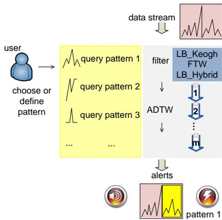
**Figure 1: Pattern detector workflow:** the user specifies query patterns which are continuously checked against the data stream using DTW lower bounds and ADTW for efficient processing. Detected patterns results in visual and audio alerts and highlighted areas in the stream.
