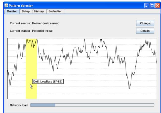
**Figure 2: Monitoring screen with alert information:** displays the currently observed data stream source, its threat status, as well as the life stream situation.
