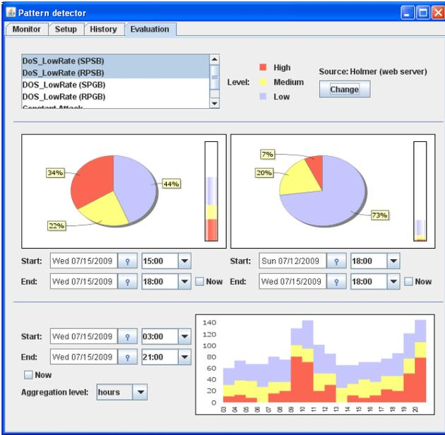
**Figure 3: Statistics screen for (historical) analysis:** allows for in-depth analysis of a specified data stream source for different patterns and periods of time, aggregated to the desired time granularity level.
