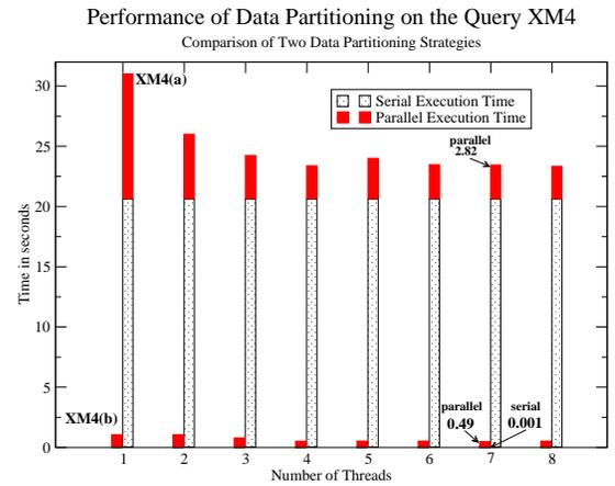
**Figure 7: Data Partitioning of the query XM4 using two different partitioning strategies. The left stacked-bar represents the performance of XM4(A), the right stacked bar represents the performance of XM4(B).**
