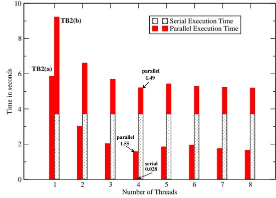
Figure 14: Data partitioning of the query TB2. The left stacked-bar represents the performance of TB2(A), whereas the right stacked-bar illustrates the TB2(B) performance. The TB2(B) performance gets affected by the large serial costs, reducing its scalability (1.73 for 4 threads). TB2(A) results in a scaleup of 3.73 for 4 threads.
