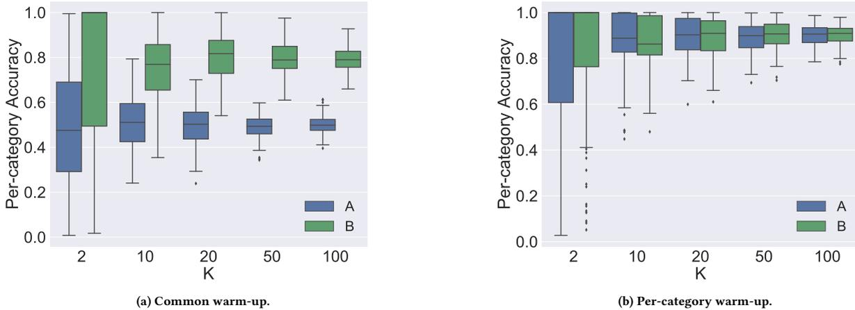
**Figure 5: Per-category accuracy of Algorithm 2 as a function of  $K$ , on a balanced synthetic dataset of size  $N = 10,000$  with average constraints. Category A items in the input have strictly lower scores than category B items. A common warm-up period leads to lower accuracy for both categories compared to per-category warm-up periods, and places items in category A at a particular disadvantage.**
