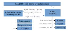
Figure 1: The software architecture
