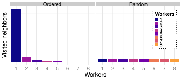
Figure 6: Visited neighbors per worker during a BFS using static partitioning on a social network graph with different vertex labelings
