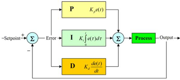
Figure 2: A sample PID controller block diagram
