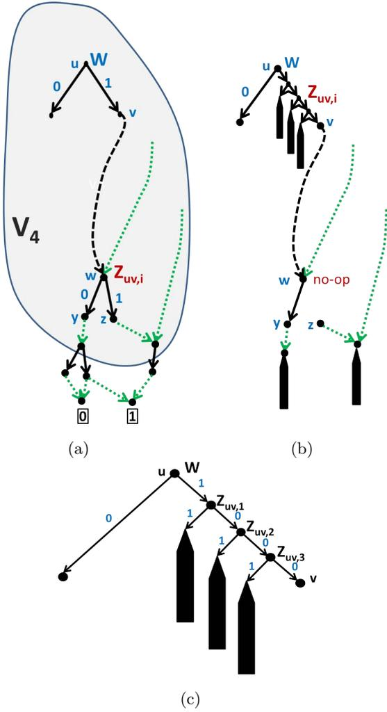
Figure 2: Given an FBDD  $\mathcal{F}$  for  $\Psi = f(\mathbf{H}_k)$  in (a), apply the conversion to produce  $\mathcal{F}'$  for  $\mathbf{H}_k$  as in (b), with detail for unit propagation in (c) in case that setting  $W = 1$  produces new  $\mathbf{H}_k$ -units.
