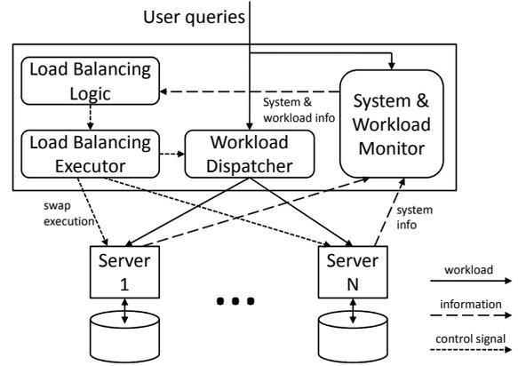
Figure 2: System Architecture
