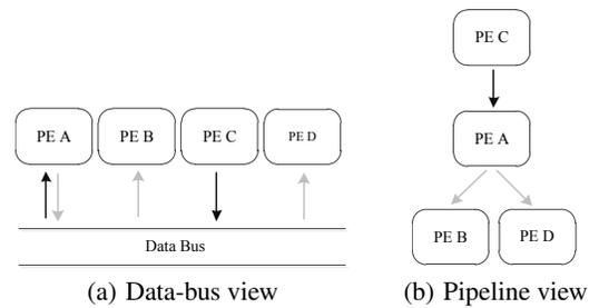
Figure 1: Data-bus view and pipeline view of the S4 event flow
