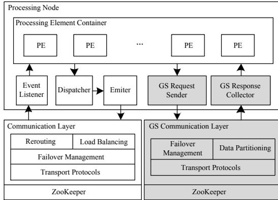
**Figure 6: The modified processing node in Pollux: the global storage components are marked with shaded background**
