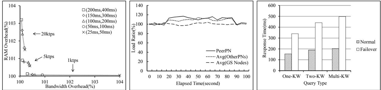
(a) Runtime overhead for varying slot-reconciliation interval and latency threshold values (b) Load dispersion during recovery (c) Response time of queries: running normally vs. resumed after failover
