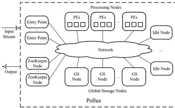
**Figure 2: Pollux’s architectural overview: processing nodes, global storage (GS) nodes, entry points, ZooKeeper nodes, and idle nodes**
