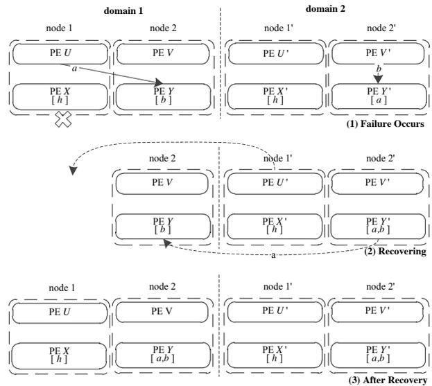
**Figure 4: A typical failure-recovery process (illustrated with two domains): (1) PE  $U$  is about to send event  $a$  to PE  $Y$  when failure occurs to node 1; PE  $U$ , PE  $X$  and event  $a$  are lost; (2) node 1' replicates its internal state to the new node 1, and PE  $Y'$  remedies event  $a$  to PE  $Y$  via slot-reconciliation; (3) after recovery, no data is lost.**
