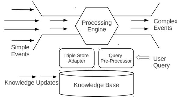
**Figure 1: High Level Architecture of Semantic-Enabled Complex Event Processing**
